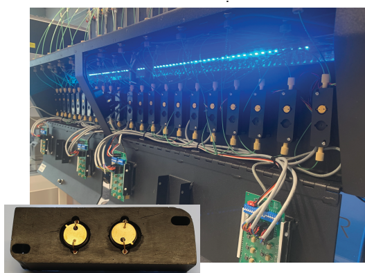
24 individual flow cell blocks for independent monitoring of each sample
